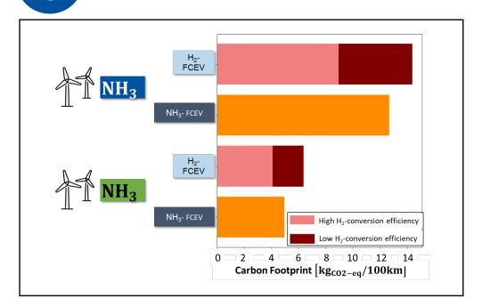
Jsage of  $NH_3$  in fuel cells can reduce CF more than usage of  $NH_3$  as a transport vector
