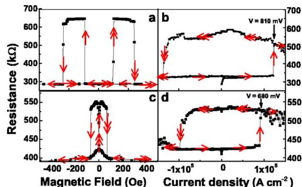
FIG. 3. (Color online) (a) Resistance versus magnetic field at 3 K and 20 mV. (b) Resistance versus current density at 3 K (initial temperature at low current density) in a field of 13.5 Oe (the initial state has parallel magnetizations in the positive field direction). (c) Same as (a) but at 30 K. (d) Same as (b) but at 30 K.
